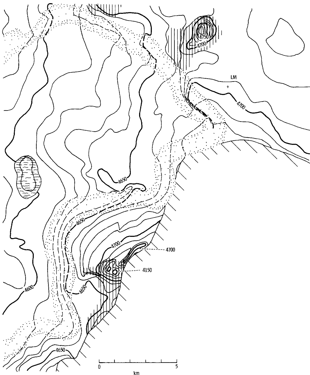
FIGURE 25-46.—Map of part of Hadley Rille (stippled area) near the Apollo 15 landing site. The area is outlined in figure 25-47. In the mare area, contours (in meters) are generalized from a 1:25 000-scale map (fig. 25-35(a)). The contours are extrapolated across the rille as dashed lines to contrast elevations and slopes on either side of the rille. Vertically ruled areas are dark, low hilly regions, which were shown on premission geologic maps (ref. 25-15) as hilly material coated by a dark mantle. Slant hachures indicate Apennine massif. Wavy horizontal pattern indicates materials of a crater doublet of probable volcanic origin.
