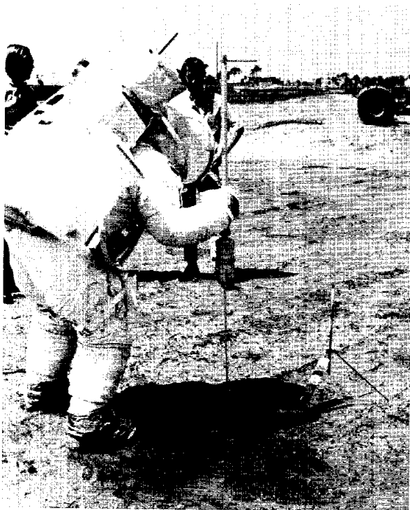
FIGURE 7-2.—Self-recording penetrometer in use during premission simulation.
