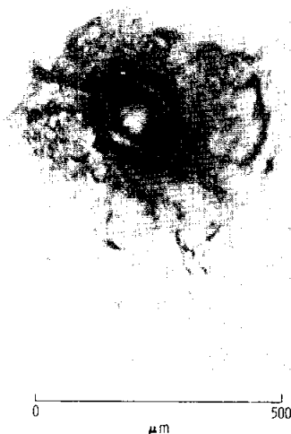
FIGURE 24-3.—Suspected meteoroid impact crater found on the Apollo 13 right-hand side-window surface.
