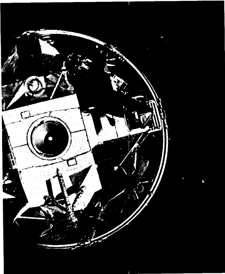
FIGURE 3-2.—During the translunar-coast phase of the mission, the CSM completed a transposition and docking maneuver to extract the LM from the SIVB stage. The top hatch and docking target on the LM are clearly visible in this predocking photograph (AS15-91-12333).
